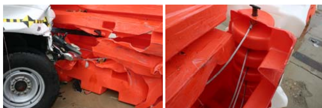
Four Cables, Preventing Vehicle Breaching
