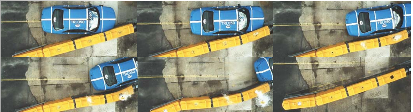
Tested and Passed: EN1317-4 P4 Impact Speed: 110 Km/h Vehicle Type: 1500 kg Bullet Vehicle Impact Angle: 15° Side
