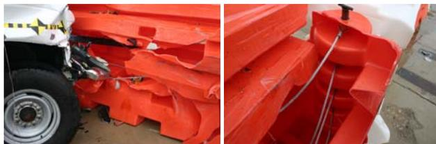
Four Cables, Preventing Vehicle Breaching
